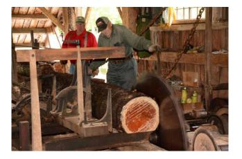
Also driven by the main drive shaft were the belts and pulleys that supplied power to reverse the carriage once the log had passed through the saw. The saw operator would pull a lever to reverse the carriage and return the log to the starting point where it could be repositioned and readied for the next pass through the saw.
