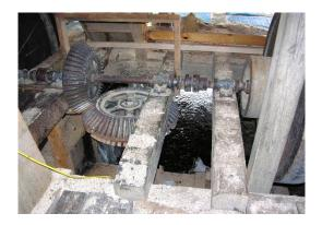
The main component of the mill powered by the main drive shaft was the main saw (or headrig) in the mill which could be either an "up and down" saw or "circular saw". Another critical item controlled by the same shaft as the saw was the carriage (the moveable rack on which the log sat to be fed through the saw). The only way to shut down the main saw was by closing the gate and shutting off the flow of water.
