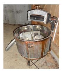
The Easy Washer boasted an all copper wash tub, steel frame, cast aluminum and brass parts and a Westinghouse electric motor. Contrast this with the early wash board and the later manual "dollie" type illustrated previously.
