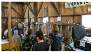
The class lines up to try their hand with the old crank corn sheller. This corn sheller was manufactured in Boston, MA by Nourse & Co. The unshelled corn was placed down the small chute at the top as the crank was turned. The interior mechanism would shell the corn from the cob and drop the kernels to a receptacle placed below and the cobs were expelled through the opening in the end.
