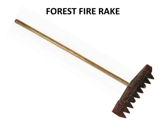
A fire rake is a wildland fire fighting tool with a rake head consisting of very sharp, serrated, triangular steel teeth. It is used to rake a fire break with the sharp teeth enabling it to reach fire in undergrowth and to loosen surface debris.
