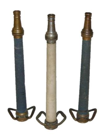
Early in the 19<sup>th</sup> century the fire service discovered that long pipes with a smooth interior created straight streams of water. These playpipes evolved from a general-use firefighting hose nozzle to a specialty tool for inspectors to measure how quickly water flows when testing hydrants, pumps, etc..
