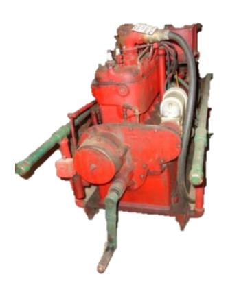
This pump is powered by a four cylinder automobile engine mounted with it. Even with four men it must have been unbearably heavy in rugged terrain.
