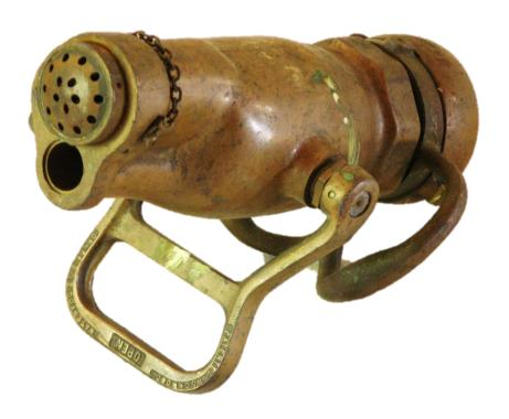
Combination Nozzle - Navy Nozzle made by the Rockwood Sprinkler Company in Worcester, MA. These are commonly referred to as shipboard firefighting nozzles or navy nozzles. Its official name is a "Rockwood Waterfog". The position of the handle gives either a fog stream or a straight stream.
