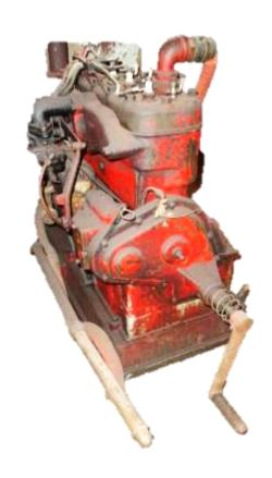
Another example of a four cylinder auto engine being mounted on rails so that it could be carried by four men into remote areas to provide power for pumps, generators, and other equipment.
