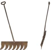
When engaged in a large cutting of ice they use a scorer such as this to mark out lines on the ice which the workers would follow when cutting free the ice blocks.
