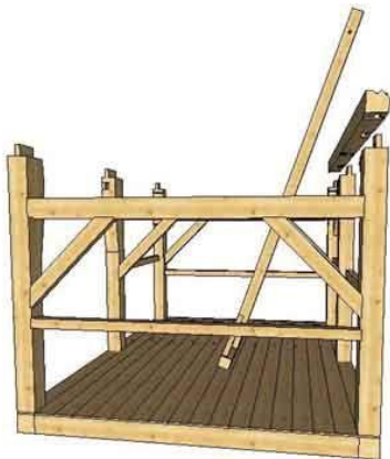
GIN POLE WORKING FROM UPPER FLOOR
