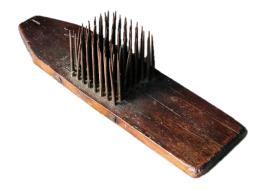
The hetchel (a/k/a hackle) is a board with a bed of nails used to comb the flax fibers after scutching\*. The hetchels were fastened to a surface in a series from coarse to fine. A bundle of flax fiber was flipped over the teeth and pulled through. Doing so separated the fibers from the flax plant in order to spin it into linen thread.
