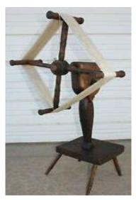
A simple device that by turning the wheel 40 times, wound approximately 80 yards of yarn into loops with which to form a skein.
