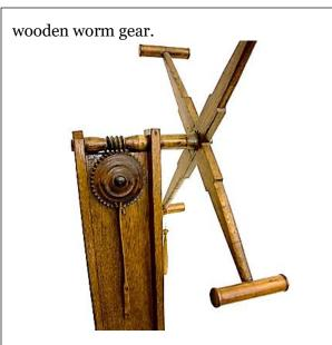
As the gear turned a small wooden peg would come against a wooden reed causing it to bend and snap back into place creating a loud "pop". This would alert the spinner that they had reached the 40<sup>th</sup> revolution and the 80 yards of yarn were complete.
