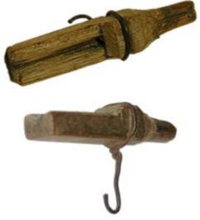
Looking closely, the work that went into a single spile is clear. The squared spout with the channel down the middle, the curved groove around the entire spiel to hold the bucket in place, the rounding and tapering of the end that will be driven into the tree and the small hole (not visible) that leads from the channel all the way back through the end that is driven into the tree.
