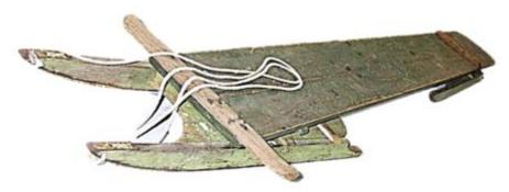
The toboggan sled was little more than a board with a set of sled type runners under the back and another set of runners under the front. The front runners were affixed to a small platform between the two runners. The only thing holding the long board of the toboggan to the front runners was a single steel pin that fit into a hole in the platform (colored yellow for illustration).
