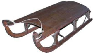
These first sleds had wooden runners. They did not track well and were hard to steer. As mentioned, the farm equipment manufacturers were skilled in combining both steel and wood into finished goods and soon steel runners were added.
