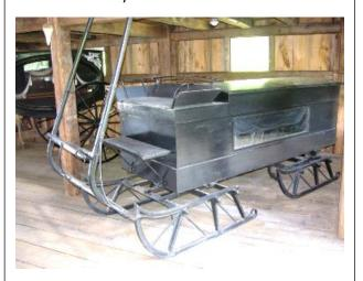
This winter hearse was built ~1870. The four wooden skids have metal strips along the bottom to prolong the life of the skid and prevent wear. The coffin slides in and out on rollers and the hearse floor elevates the coffin off the rollers to prevent the coffin sliding during travel.
